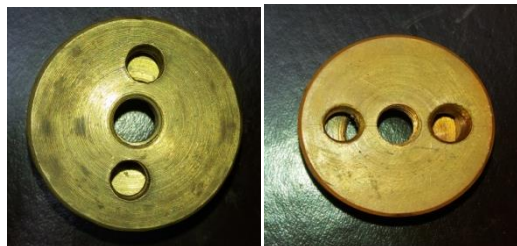
Fig 4.8.1 Hot end (Brass and Copper)
