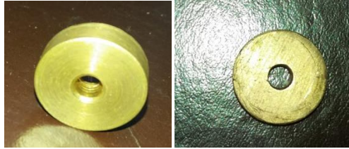
Fig . 4.6.1 diaphragm (Copper and Brass)
