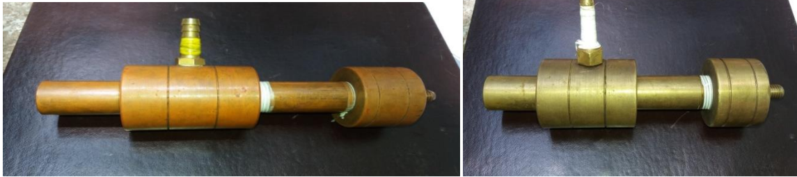
Fig. 4.9.1 vortex tube assembly (Copper and Brass)
