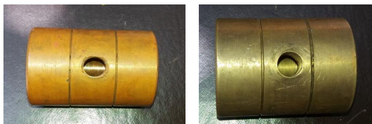
Fig. 4.2.1 Main body (Copper and Brass)
