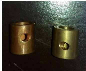
Fig . 4.7.1 nozzle (Copper and Brass)
