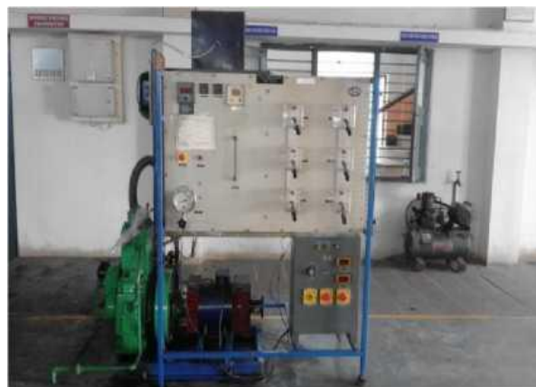
Figure 2: Four stroke single cylinder diesel engine set up with generator loading
