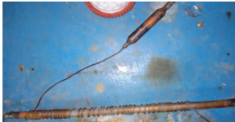
Figure 3 Heat Exchanger like set up
