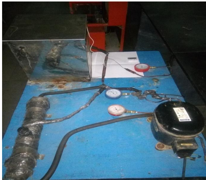
Figure 4 Complete set up with Heat Exchanger
