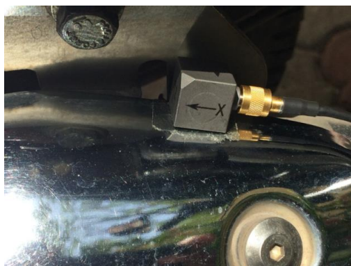
Figure 16. Accelerometer put on silencer
