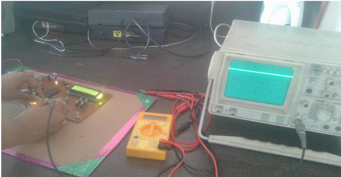
FIG.7:-Output Magnitude Test of Dc-Dc Boost Converter on CRO
