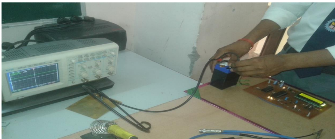
Fig.6:-Input Supply Test Waveform on CRO
