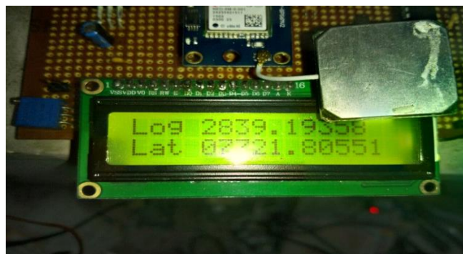
Figure 4. LCD shows the longitude and latitude position locked by the GPS receiver.
