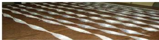
Figure 8: Varying length twisted tape
