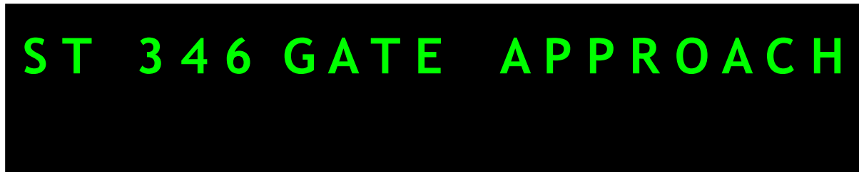
Figure 7: Loco Pilot Display before 2000mt of approaching gate
