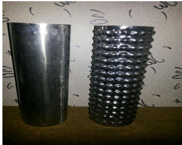
Figure 12: Plain and Modified body of silencer
