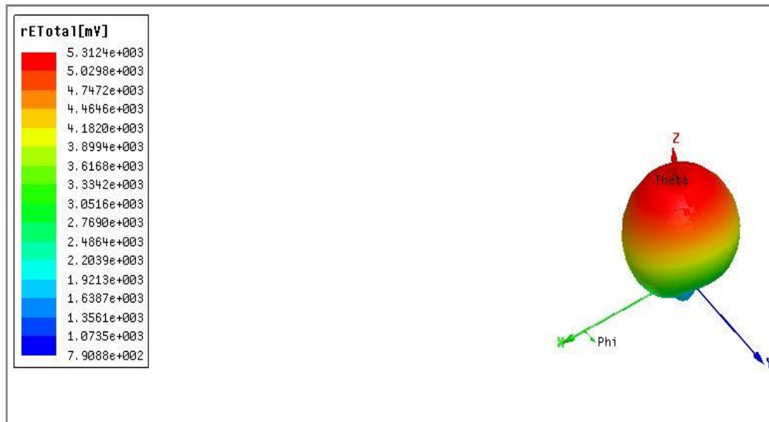
FIG. 5. 3D RADIATION PATTERN.
