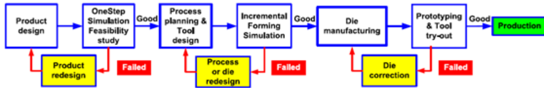
Fig.No.6 The work flows in simulation based process planning and die design
