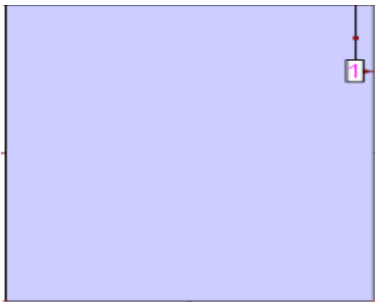
Fig.2 Rectangular Patch without Slots
