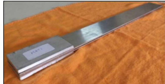
3(b) Symmetric sandwich CLD beam
