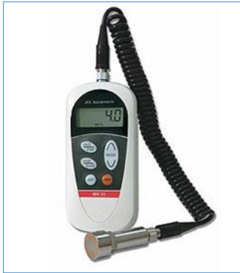
Figure 4: Typical vibration sensor device for FFT analyzer
