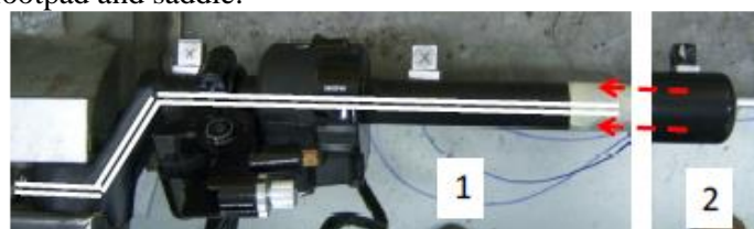
Figure 2: Handlebar; (1) fixed beam, (2) insertion of steering balance into extremity of handlebar.
