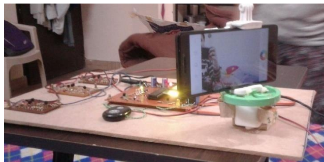
Fig 10: Rotor rotates and captures the snap in the desired direction.
