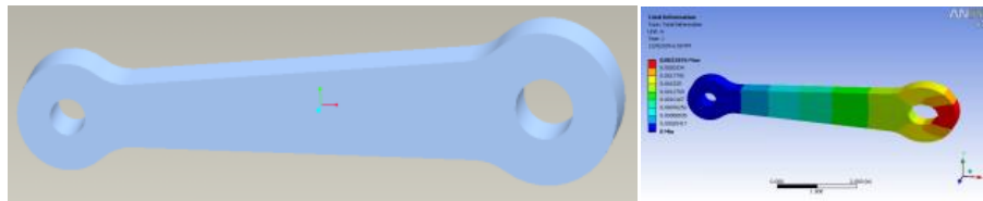
Fig. 3(b) link 2 design and simulation results
